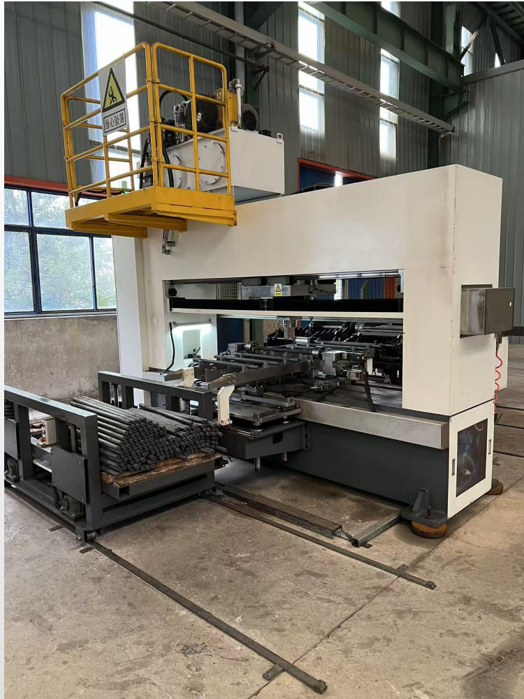
Automatic drill rod straightening machine
